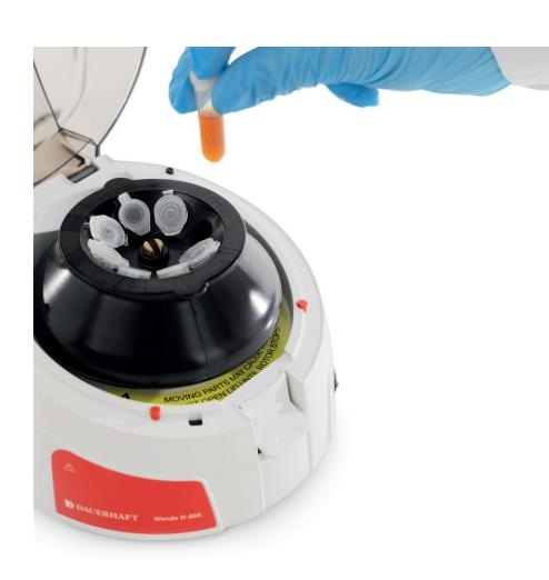
Rotor for 8 microtubes
